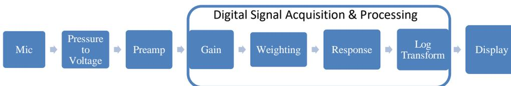
*Figure 1.* Sound level meter signal processing chain.
